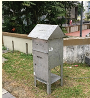
Air Quality Monitoring by using High Volume Sampler
